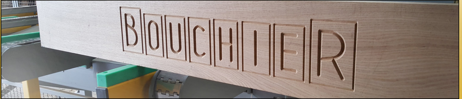
Engraved Oak beam on Hundegger SC3 machine
