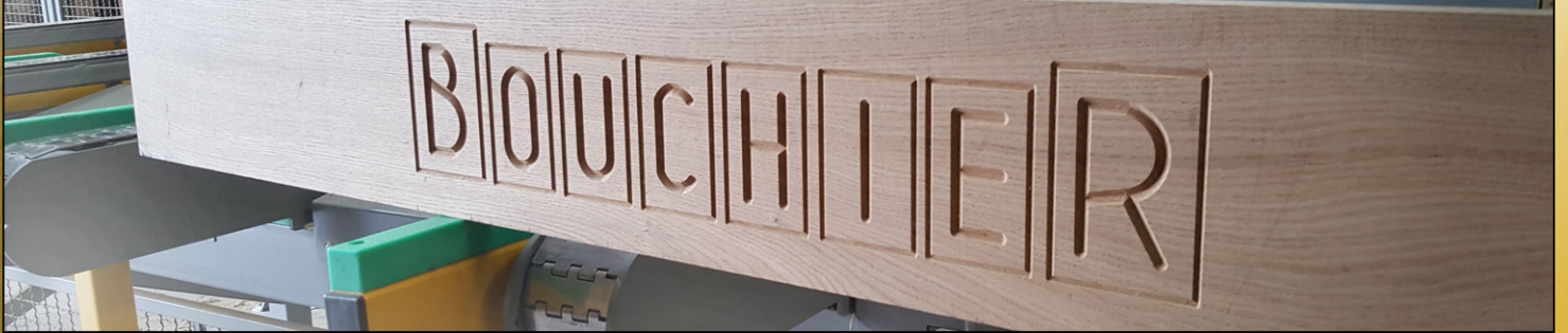
Engraved Oak beam on Hundegger SC3 machine
