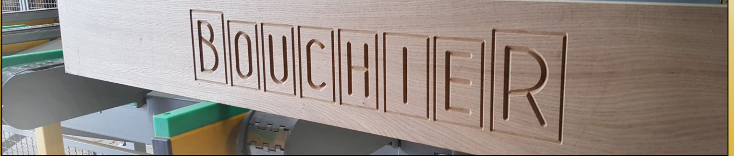
Engraved Oak beam on Hundegger SC3 machine
