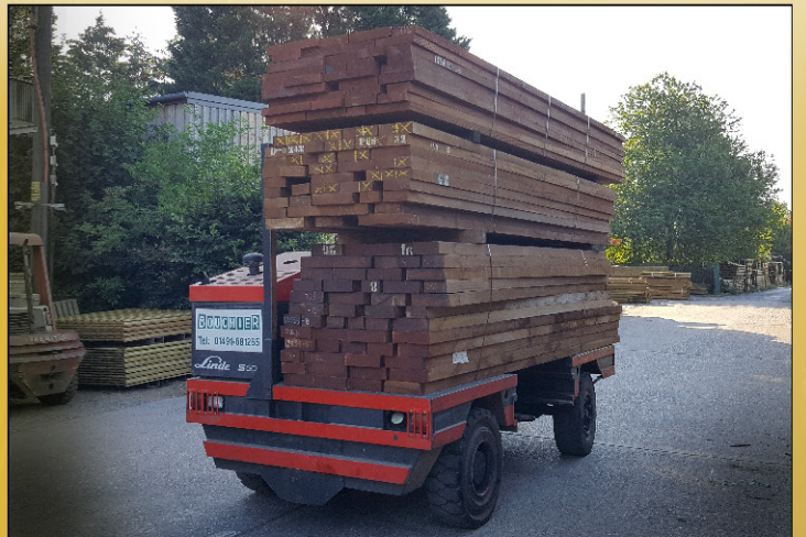
Iroko prior to machining for Entrance Gates
